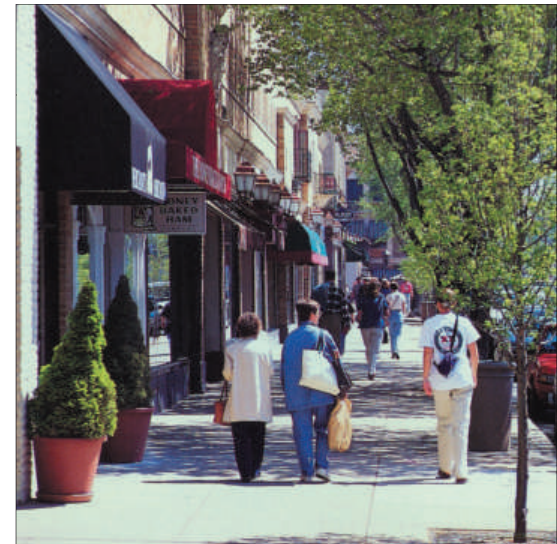
Sidewalks should be subdivided into three zones: a clearly defined curb zone for planting and furnishings, an unobstructed pedestrian circulation zone, and a few objects placed against the building wall in the building zone.
